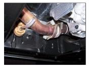
1. To remove the stock exhaust remove it from the 2-bolt flange located in front of the stock muffler. Disengage the welded hangers using WD-40 from the OEM rubber grommets. Do not discard, damage stock bolts or remove the rubber grommets as you will re-use them to mount your new system. Now, cut off tailpipe and remove exhaust.
