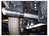
**5** Next, install the exit pipe #D to tailpipe. Use clamp #F to secure. DO NOT TIGHTEN. Insert welded hanger into rubber grommet.
